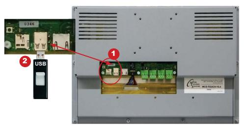
On back of touchscreen, locate the USB PORT as shown on screen 1 and insert a USB stick to copy necessary files. There are two USB ports,
